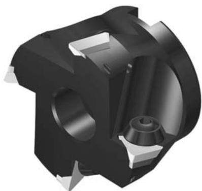
**Characteristics:** This positive milling cutter with an exact angle of 90° uses very strong inserts allowing depth passes and high feed per teeth. The damp allows a quick insert assembly and dismantling. The milling cutter is equipped with shim seats (except diameter 40 and 50 mm), which protect the milling cutter body in case of accident. Axial rake=+6°; Radial rake=+1°.
