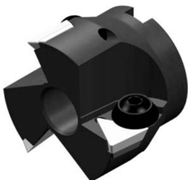
**Characteristics:** This positive milling cutter with an exact angle of 90° uses very strong inserts allowing depth passes and high feed per teeth. The clamp allows a quick insert assembly and dismantling. The milling cutter is equipped with shim seats, which protect the milling cutter body in case of accident. Axial rake=+6°; Radial rake=+1°.
