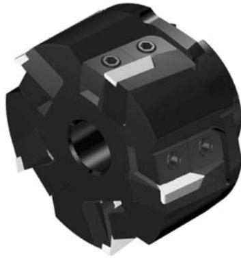
**Characteristics:** This positive milling cutter with an exact angle of 90° uses very strong inserts allowing depth passes and high feed per teeth. The fixing system by wedge ensures an excellent clamping of the insert and a higher security on difficult conditions. The indexable cartridges protect the milling cutter body in case of accident. Axial rake=+7°; Radial rake=-1°.
