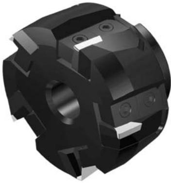
**Characteristics:** This positive milling cutter with an exact angle of 90° uses very strong inserts allowing depth passes and high feed per teeth. The fixing system by wedge ensures an excellent damping of the insert and a higher security on difficult conditions. The indexable cartridges protect the milling cutter body in case of accident. Axial rake=+7°; Radial rake=-1°.
